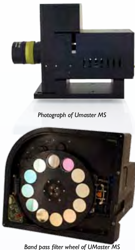
Band pass filter wheel of UMaster MS
