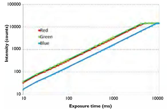
Linearity of the iSENSE-Color measured for the R, G and B pixels
